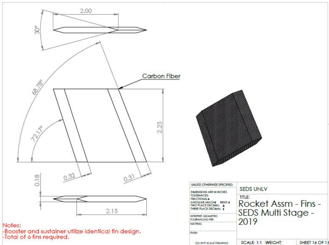
Figure 3: Fin Design Drawing
