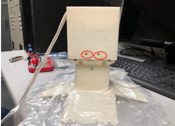
Figure 3: Screw location adhering Cube 2 to Cube 1.
