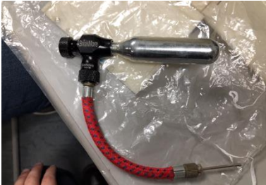
Figure 5: Canister correctly fastened to valve
