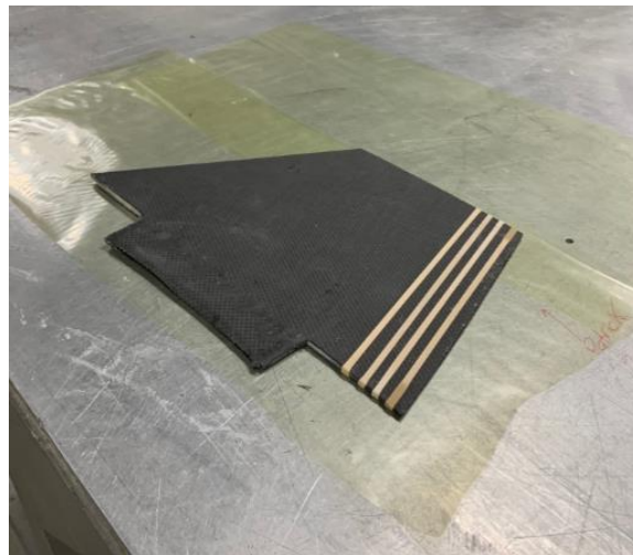
Figure 10: Finalized Composite Fin
