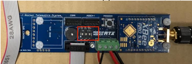
Figure 14: Dip switch settings set to ON, ON, ON for the Base RT x module.
