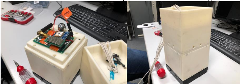
Figure 8: Placing of the telematics device before covering with Cube 2
