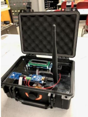
Figure 22: Recovery Team Ground Station
