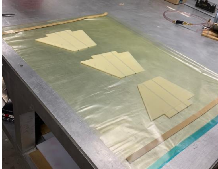
Figure 8: Start of 3D Printed Fin Layup
